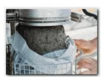
phase - weight of sludge 70-80 kg ( 20% dry solids), after two months, a cake of at least 50% dry solids content. This would weigh only 35 - 40 kg and represents almost a 50-fold reduction of
